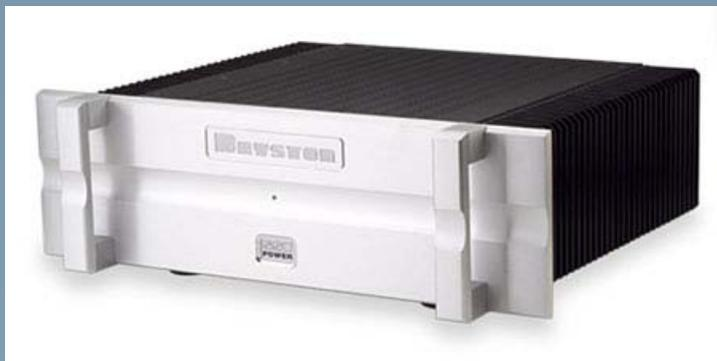
The superbly built 7BSST2 offers 600W in fully balanced, class A1/B operations into 8 ohms, and features a dual-mono bridged circuitry in which the two amplifiers modules in each monoblock chassis are wired in series and driven by opposite-polarity signals, Changes from the original 7BSST include a circuit
