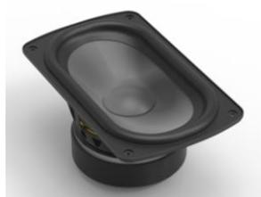
The newly engineered 6"x10" active low-frequency drivers for the built-in powered subwoofers have 40% more surface area than the active drivers used in the Triton One, along with a larger diameter voicecoil and an even more massive magnet structure which also utilizes our "Focused Field" technology.
