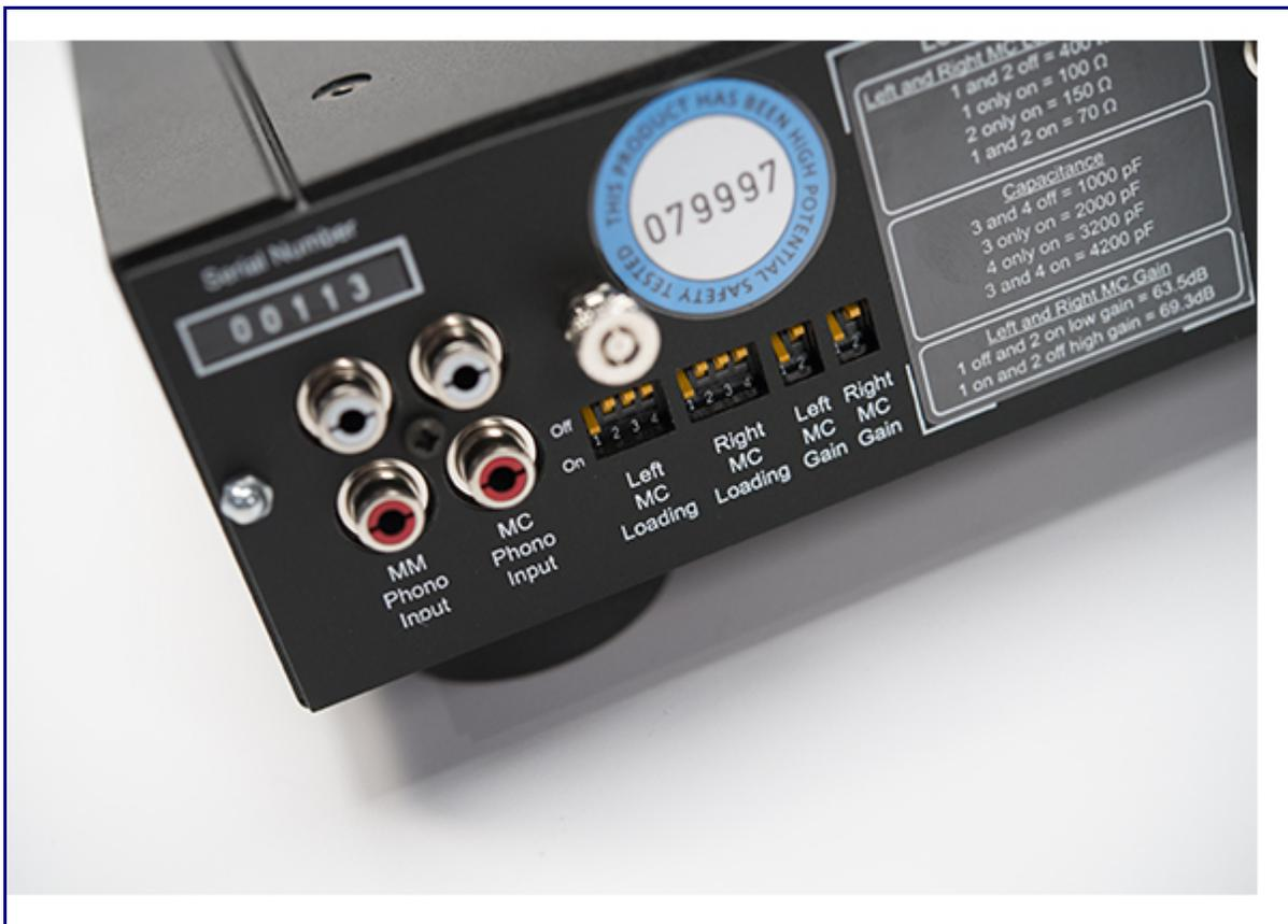
The compact physical size of the Aria is unobtrusive, keeping the same form factor as Rega's current Brio-R integrated amplifier, Apollo-R CD Player and DAC. The rear panel has two pairs of RCA input jacks, one for MM and one for MC phono, with a pair of RCA output jacks to connect to the rest of your system.
