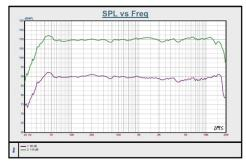
Above, note that the frequency response of the speaker at a punishing 110dB is virtually identical to that of the speaker at a more common level of 90dB. This is astonishing performance regardless of price.
