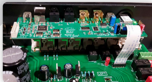
DA200 DAC board on IN100 Signature.
